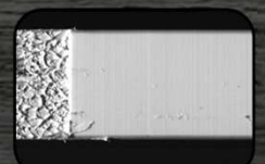
Missing edge band / band gap
